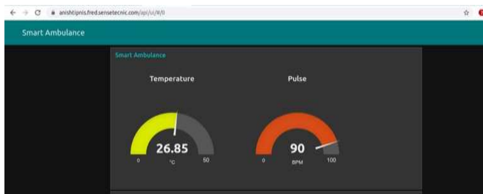
Fig. 4 : Gauge view of temperature and pulse on the Node-RED dashboard
