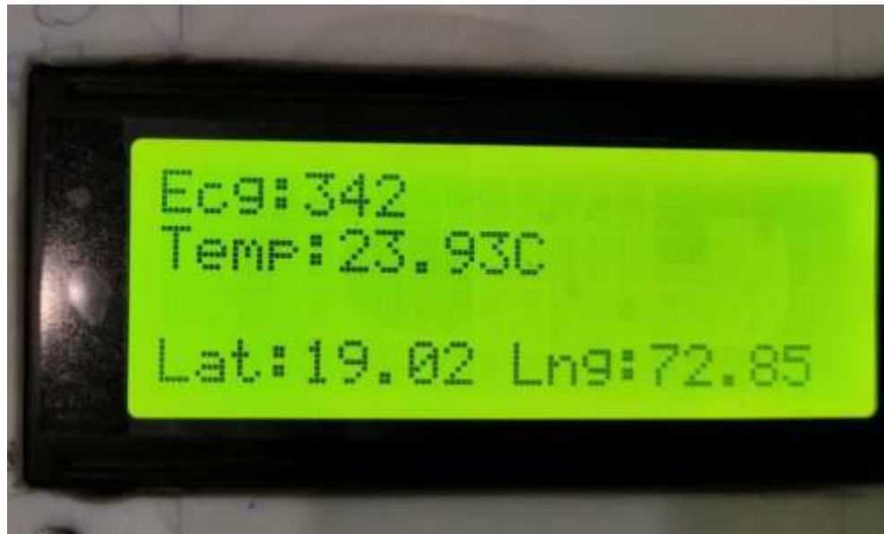
Fig. 2 : LCD output of the values from sensors and location of ambulance.
