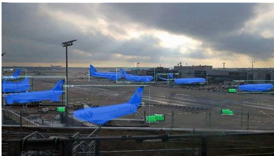
An example of how a computer identifies aircraft (blue) and other ground vehicles (green). This system can also be used to avoid collision with other automated ground vehicles.
